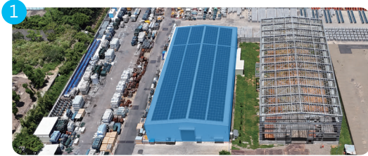
Heavy electric plant/finished product warehouse roof Solar panel installation capacity: 392kW
